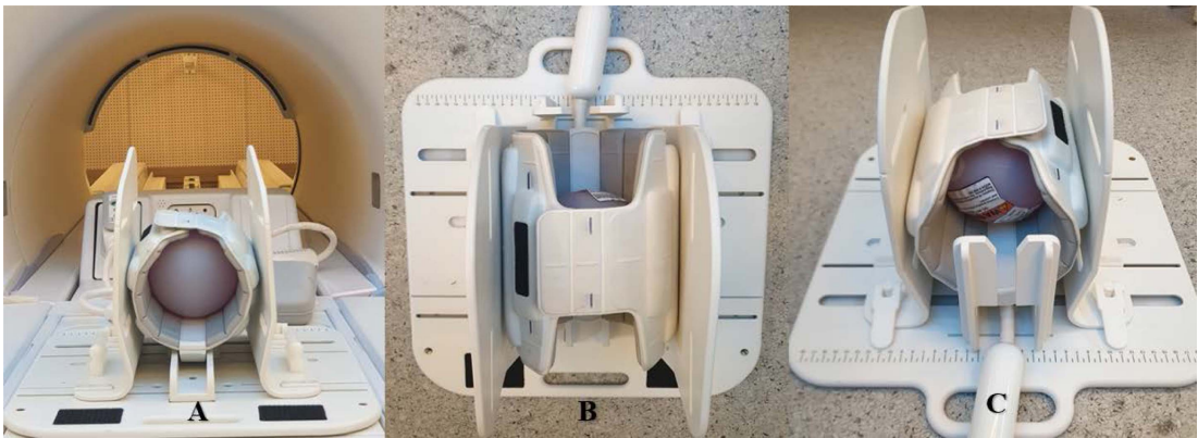
Fig. 4. (Color online) Arrangement of spherical phantom, fixed frame (A), and coil with surface coil wound (top view B, front view C).
