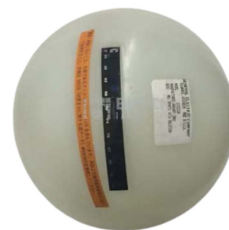
Fig. 2. (Color online) MRI-specific phantom for image quality evaluation (including MRS 4.38 Sphere solution phantom).
