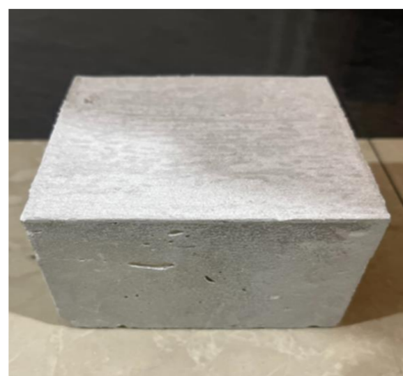
Fig 6. Cement barium sulfate shield (6cm)
