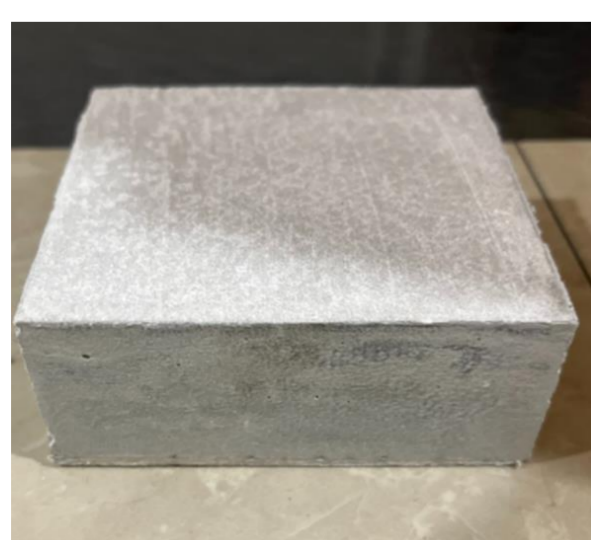
Fig 5. Cement barium sulfate shield (4cm)
